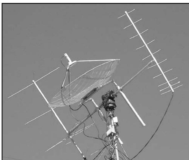
Fig 50—The 1.2-meter dish with dual-band patch feed installed. ( K5OE photo; courtesy of The AMSAT Journal. )
