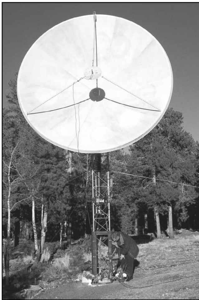
Fig 26—W0LMD found the ultimate in this 14-foot dish for AO-40, with a triband patch feed and Az-EI mount. (W0LMD photo.)
