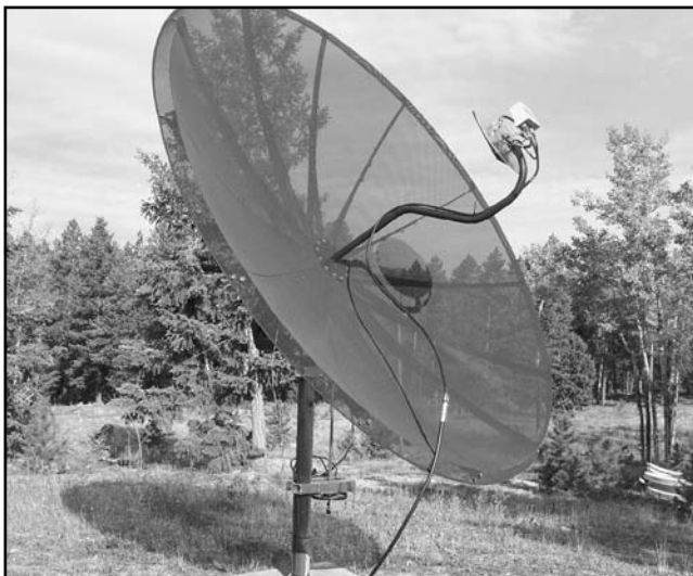
Fig 25—W0LMD increased to this 10-foot dish for AO-40 operations, with a triband patch feed for U, L, and S bands on an Az-EI mount. (W0LMD photo.)
