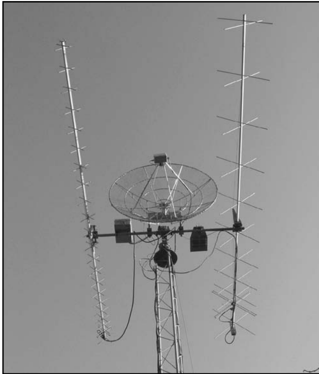
Fig 22—Wilfred Carey, ZS6JT, constructed this cluster of satellite and EME antennas. Left to right: 2 × 23-element offset feed Yagi for U band; 1.64-meter dish with 2\frac{1}{4} -turn helix feed for S band; 2 × 11-element coplanar feed Yagi for V band. (ZS6JT photo.)
